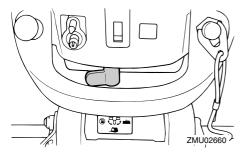
5. Tilt support bar equipped models: Hold the rear of the top cowling or the rear handle (if equipped) with one hand and tilt the outboard motor up fully until the tilt support bar automatically locks.
